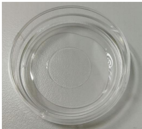
Figure 19. Nonporous PET membrane as a printing substrate. The membrane was punched with a 15 mm puncher and placed onto a culture dish. After printing, 300 – 400 µl of Cnt-30 medium or 1X PBS was added to the edges of the dish to provide humid environment for the hydrogel and prevent it from drying.
