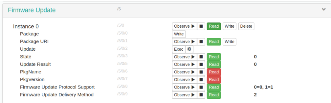
Figure 6.12. Read operation performed on firmware object
