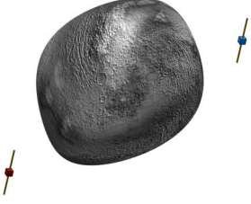
Fig. 1. Two small spacecraft exploring the interior of an asteroid. Each one is equipped with a single-rod dipole antenna similar to those utilized in low-frequency georadar surveys.
