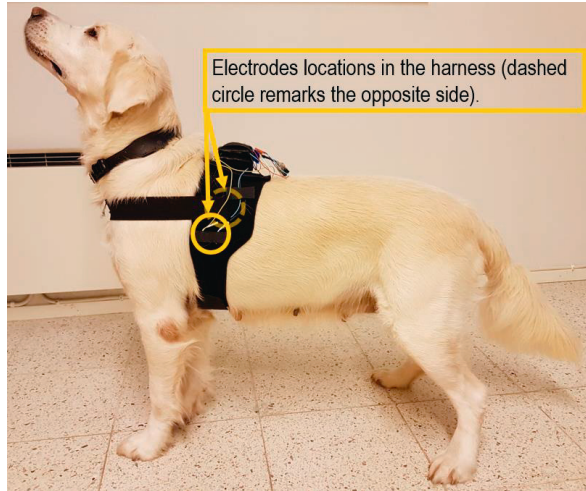
Figure 17. The ECG measurement harness dressed on a dog with electrode locations marked with yellow circles.
