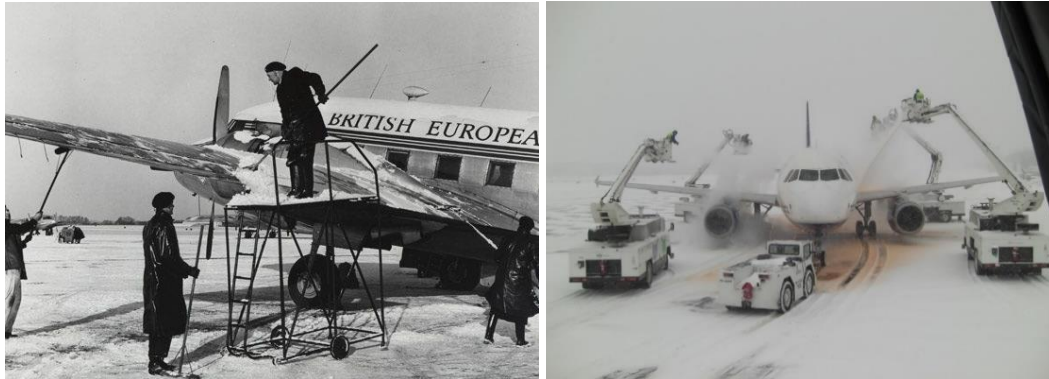
Figure 4. Photographs of current and historical de-icing methods for the removal of ice off aircraft wings [12].
