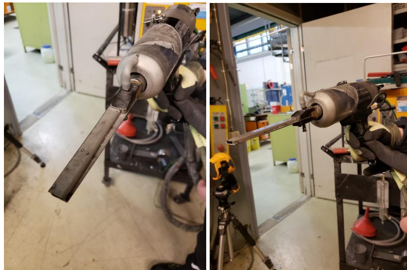
Figure 48. LPCS gun nozzle showing modified nozzle with rectangular shape
