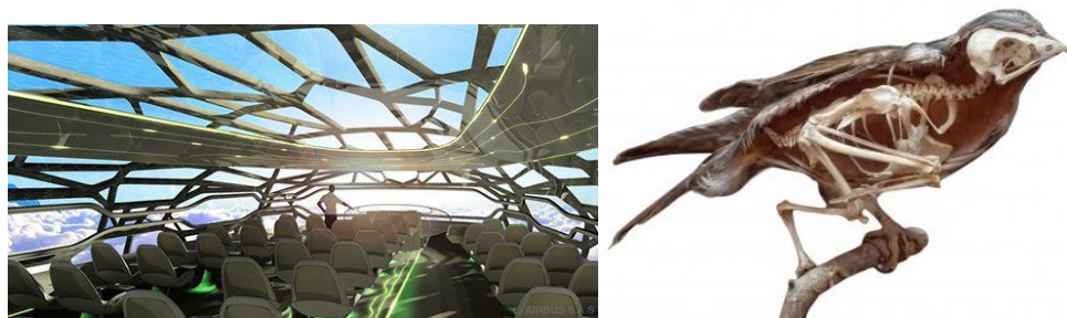
Figure 16. Airbus's 2050 aircraft structure ("bionic bone design") in comparison to a bird's porous bone structure [56],[57].
