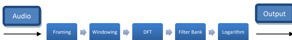
Figure 1 Block diagram for mel spectrogram calculation
