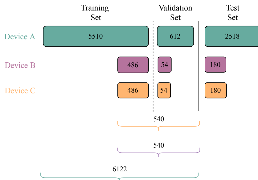
Figure 4.1. The setup of training, validation, and test splits used in our work. The numbers present the number of 10-second segments for each split and recording device.
