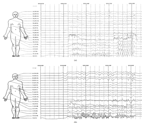
Figure 4. The estimated motion trajectories of 22 markers attached on the human body. The upper graph (a) shows their relevant motion trajectories versus time in x dimension. (b) the lower graph shows their relevant motion trajectories versus time in y dimension [40].
