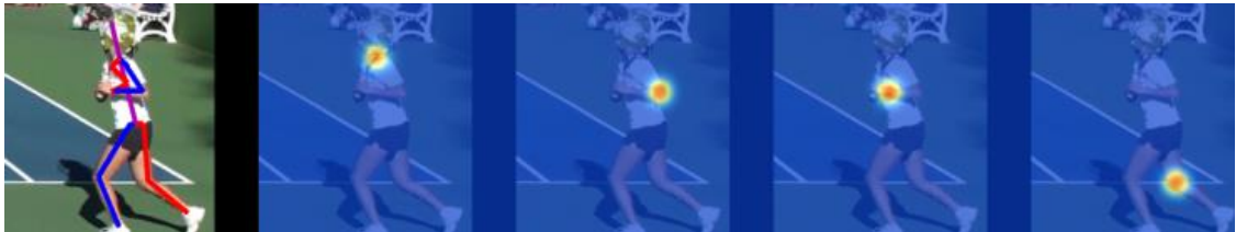
Figure 14. Output samples of the pose estimation. It constructs heatmaps to define features of the keypoints. (Images from left to right are: the estimated final pose, a heatmap of neck, a heatmap of left elbow, a heatmap of left wrist and a heatmap of right knee) [81].
