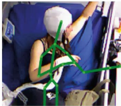
Figure 5. Motion tracking in 3D using NeuroKinect system. The skeleton estimation has not been completely accurate due to misdetection of the left arm [27].
