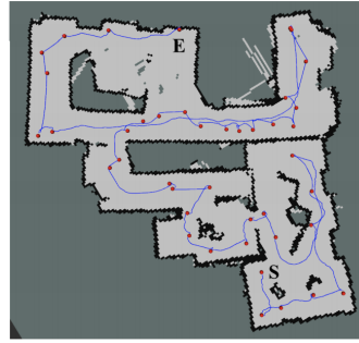
Figure 4.3. Generated occupancy grid. Occupied areas are marked black, open area is light gray and unknown area is dark gray. The line describes the robots movement from start S to end E with dots as visited frontier locations. [22]
