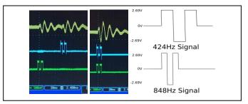
Fig. 3. Monitored view of tablet set-up via oscilloscope (on the left). Unipolar oscillograms of vibration signals have been taken from grounded resistors in a circuit of full-bridge amplifiers. Measurements recorded at 80mm from the left actuator. Example of the Haptic signal received by the Tectonic Actuator (on the right).
