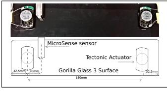
Fig. 1. Tablet set-up.
