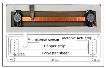
Fig. 2. Display overlay pouch sealed with liquid set-up.
