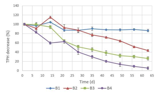
**Figure 6.4 Hydrocarbons removal during 63 days of treatment under bioreactor experiment** (**paper III**). B1: soil + sawdust; B2: soil + sawdust + mineral nutrients; B3: soil + sawdust + digestate; B4: soil + sawdust + digestate + immobilized bacteria. Results are presented as a mean of samples collected from two reactors and analyzed in triplicate with standard deviation.
