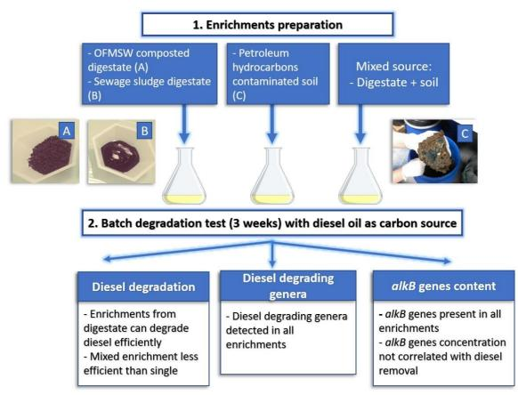
Figure 6.2 Preparation of enrichments and main outcomes of the enrichment experiment (paper I). All microbial enrichments were able to grow on diesel fuel as sole carbon and energy source. Diesel fuel degradation was observed in all flasks.
