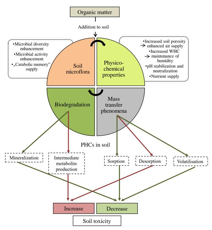
**Figure 3.1 Processes occurring after addition of pretreated organic matter to soil.** Organic matter improved soil properties and provide wide number of microorganisms including degrading agents. Humic like substances present in organic matter helps to desorb weathered contaminants as well normalize excess concentrations. Abbreviations: *PHCs* petroleum hydrocarbons, *WHC* water holding capacity.
