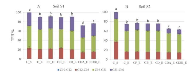
**Figure 6.3 Percentage of TPH in clay (panel A) and sandy (panel B) soil after 30 days of treatments.** C: soil + water; CF: soil + mineral nutrients; CD: soil + digestate; CDA: soil + digestate + bulking agent; CDBI: soil + digestate + bacteria immobilized on biochar; S: day 1; E: day 30. Mean (n = 3) and standard deviation. The same letters represent no significant differences among treatments for each soil, respectively (one-way ANOVA; p N 0.05).
