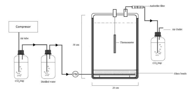
Figure 5.2 Scheme of the bioreactors used for the experiments for paper III.
