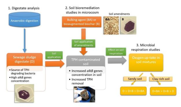
Figure 6.5 Structure and main results of microcosm experiment (paper II). The experiment examined the effect of digestate, saw dust and immobilized inoculum on PHCs bioremediation efficiency in two types of contaminated soils.
