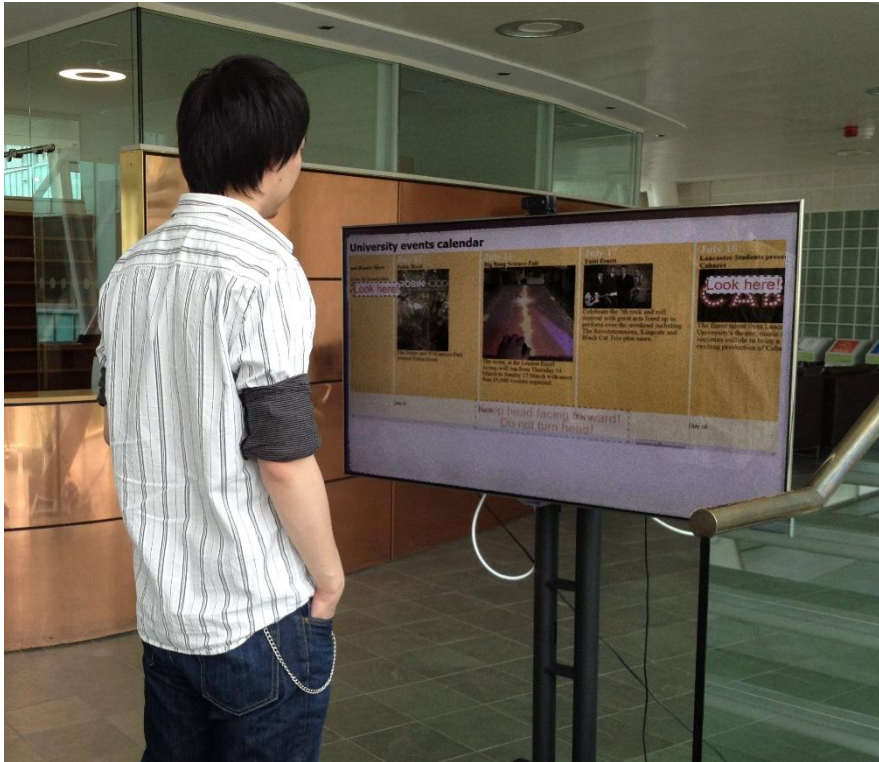
Fig 7 GazeHorizon (Zhang et al., 2015) makes any content looked at by the user drift to the center. A hint ("Look here!") is given on both sides of the screen to attract the user to glance on the side. Photo courtesy of Yanxia Zhang, 2015 (c) Yanxia Zhang
