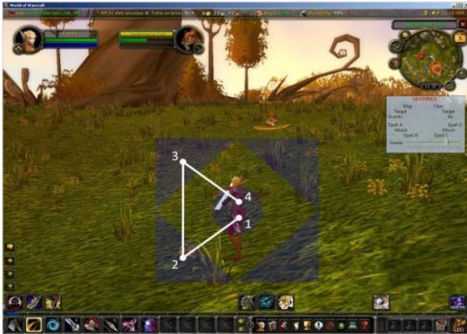
Fig. 4 On-screen gesture for gaming. The semi-transparent sectors around the avatar help the user to focus on the gaze-reactive areas. The white numbers and gesture path are for illustration only (Vickers, Istance, & Hyrskykari, 2009).
