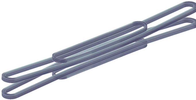
Figure 2.6 Depiction of the dipole magnet Feather-M2.
