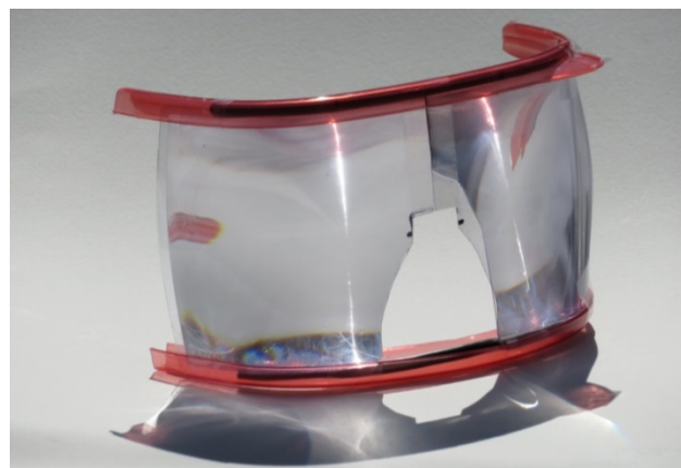
Figure 2. Super-wide-FOV curved Fresnel mask prototype
