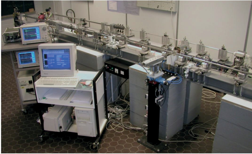
Figure 18. Photograph of the compressive split Hopkinson pressure bar equipment used in this work.
