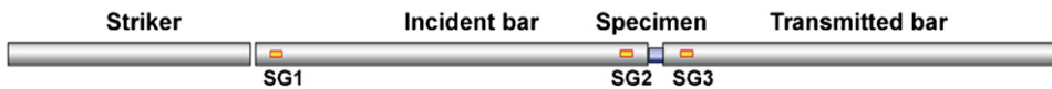
Figure 19. Positions of the strain gages in the tests of cold heading materials with extra-long strikers (Publication V).
