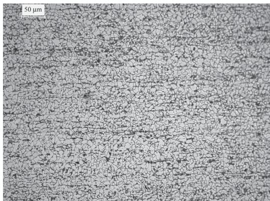
Fig. 1. Optical micrograph revealing the banded microstructure of the studied steel wire. The rolling direction is horizontal.
