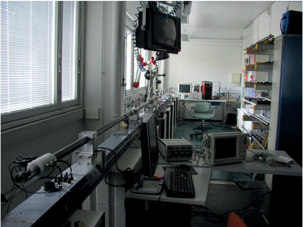
Figure 22. Photograph of the tensile split Hopkinson pressure bar equipment used in this thesis.
