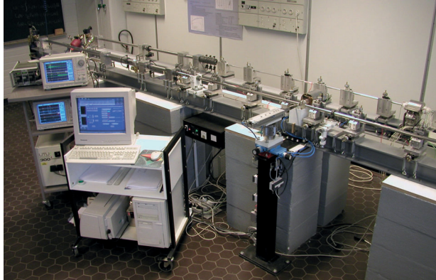
Figure 3. Hopkinson Split Bar device at the Institute of Materials Science, Tampere University of Technology.
