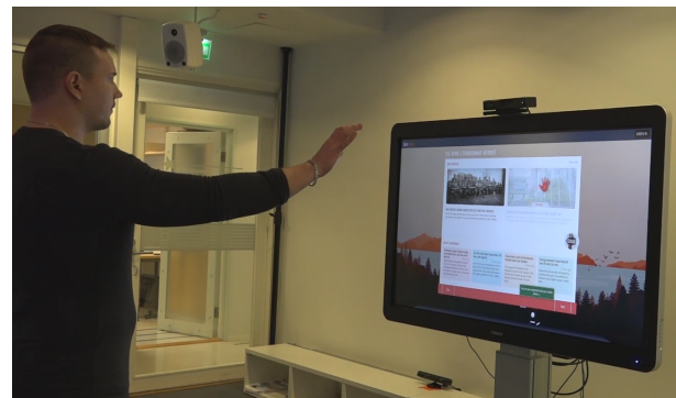
Figure 1: The SimSense system. SimSense utilizes location tracking, of both the user and the user’s mobile device, to automatically pair mobile devices with their owners. Consequently, users can pull content from the display to their mobile device from a distance, without ever touching the mobile device.
