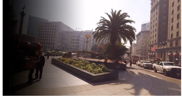
Figure 2: The Shadow Indicator . When a popular area is detected outside the view, a shadow appears on the side of the screen opposite from the popular area. In this case, the shadow appears on the left, hinting that many viewers are focusing on something to the right. The Shadow Indicator is somewhat less obtrusive on the HMD than it appears in the figure.
