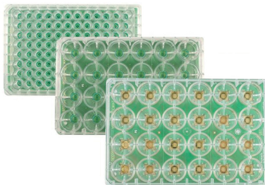
Figure 4. One 96-well (back) and two 24-well (front) and HTP MEAs by Multi Channel Systems. [Picture from www.multichannelsystems.com .]
