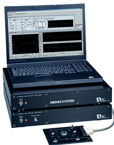
Figure 7. MED64-Basic MEA measurement setup by Alpha MED Scientific. The MEA is in the connector unit in front of the amplifier units. [Picture from www.med64.com/ ]
