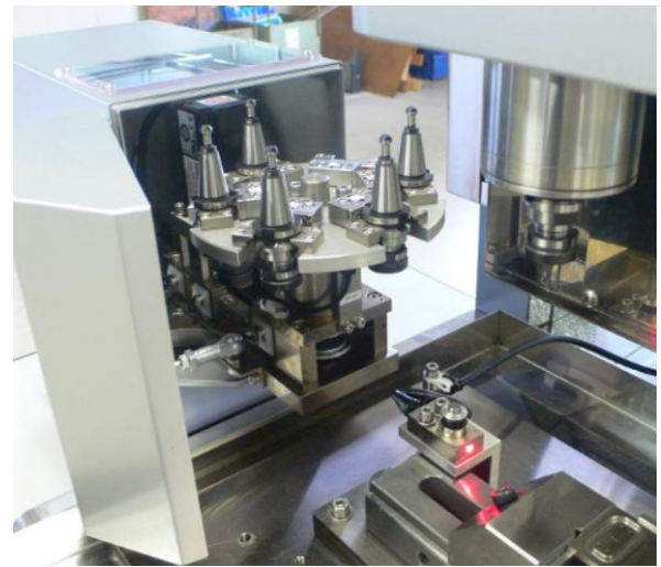
Fig. 5 ATC of milling unit-2
