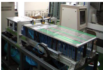
Fig. 8 Designed and manufactured inspection system with air pad
