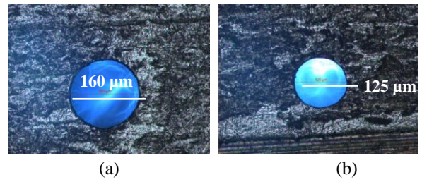
Fig. 8 Titanium, 1mm thickness, 0.1mm diameter, at top (a) and bottom (b)
