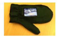
Figure 5. SeekThrough prototype: a smart phone attached to a self-made glove.
