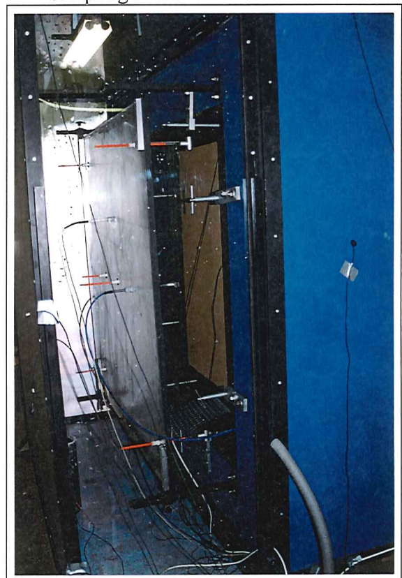
III 4. The external protective board with sensors was attached.
