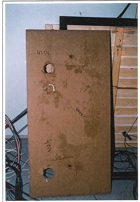
III 4. The windshield of Test Wall 2 appeared wet all over after the test.
