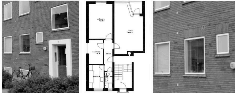
Figure 2: Natural ventilation distributed through facade related to kitchen and bath
