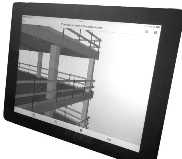
Figure 1: Structural 3D model including safety railing viewed in iPad using mobile application Tekla Field 3D.
