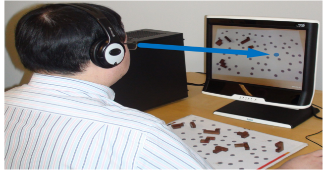
Figure 2: The setup at the instructor's end. The blue dot on screen indicated the gaze pointer. The same pointer was visible at the worker's end.
