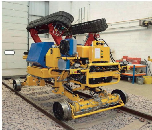
Figure 2.17. FWD developed by URS Infrastructure and Environment Ltd. for track use (Sharpe 2014).
