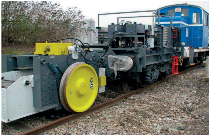
Figure 2.23. Portancemetre (Hosseingholian et al. 2011).
