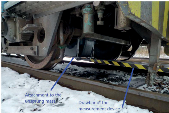
Figure 4.4. The measuring device's attachment to the TKA7's axle on the unsprung mass. A specifically designed mounting adapter is used, attached to the locomotive's transmission.
