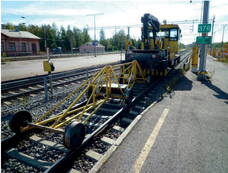
Figure 4.1. The Stiffmaster, a continuously operating measuring device for track stiffness.
