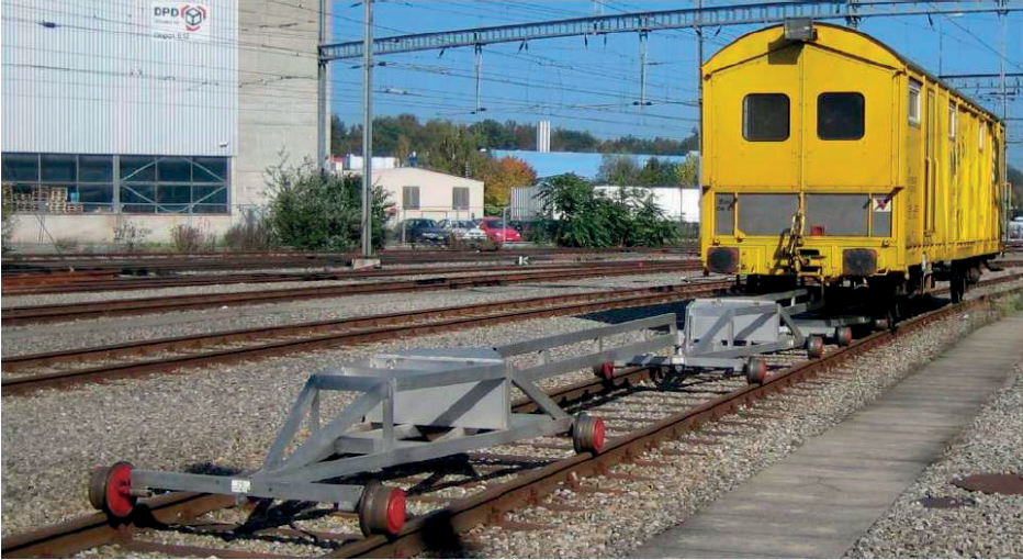
Figure 2.29. Swiss SBB's stiffness measurement system (RIVAS 2013).
