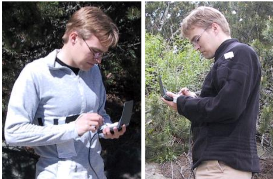
Figure 25. Second version of the heating garment prototype. On the left, the undershirt which contains all the sensors and measurement electronics. On the right, the inner covering jacket containing the heating panels and power control electronics. [Rant2_01]
