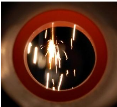
Fig. 3.2: Coal combustion under high O_2 concentration.
