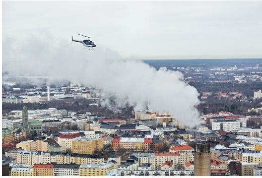
Figure 3.3: A picture of the measurement of atmospheric dilution of flue gas from pulverized-fuel combustion. Measurements were made by aerosol instruments installed in a helicopter. The figure demonstrates that the flue-gas plume can be visually observed while conducting measurements.
