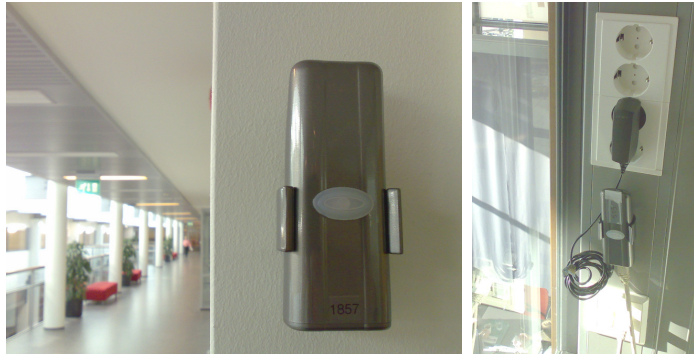
Fig. 14. Indoor deployment at Tampere University of Technology. A typical battery powered node installed at wall (left) and a mains powered sink acting as a gateway via Ethernet connection (right).
