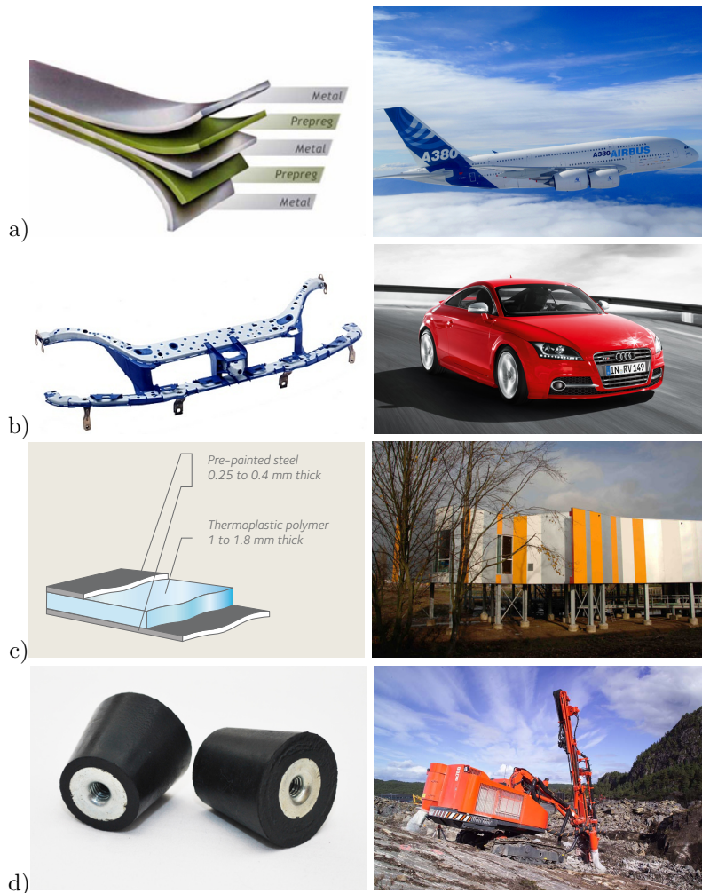
Figure 2.2: Examples of polymer/metal hybrid structures and their applications: (a) a fibre metal laminate for aeronautic applications [33, 34], (b) a polymer metal hybrid car front end [35, 36], (c) a steel-plastic-steel structure for construction applications [7], (d) a rubber/steel vibration damper for noise control and protection from forces generated in compression [37, 38].
