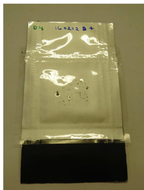
FIGURE 4.10. An example of corrosion of aluminum current collector due to poor protection by graphite layer.
