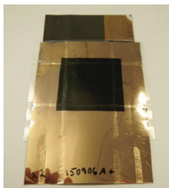
Figure 4.11. Copper frame to avoid metal corrosion and improve electrical conductivity. Adapted from III.
