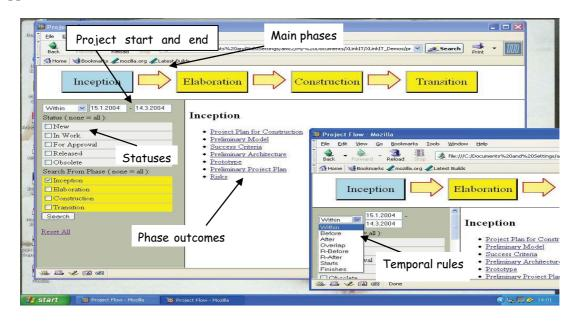
Figure 23. A dynamic project workflow chart with time-sensitive linking and navigation support
