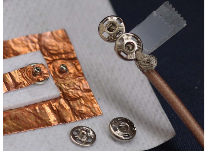
Fig. 1 Male buttons are punched through the copper foil tape, and female buttons connected by twisting the metal threads of the coaxial cable through the holes in the buttons. Loose male and female buttons are shown at the bottom.
