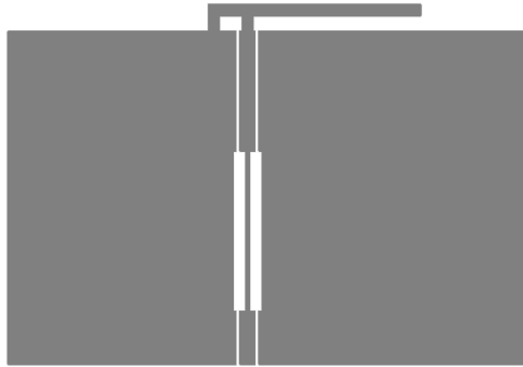
Figure 3.8: Single-layer inverted-F antenna for 1575 MHz.
