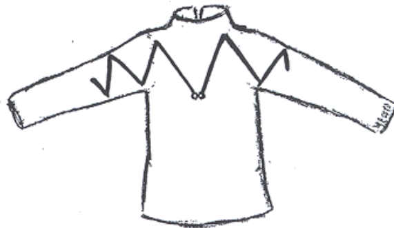
Figure 3. The meandered dipole.
