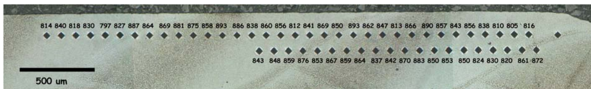
Figure 124. Optical micrograph of etched transverse (perpendicular to cladding direction) cross-section of WR6 tool steel laser coating. Reheated zones and increased microhardness values are clearly seen.
