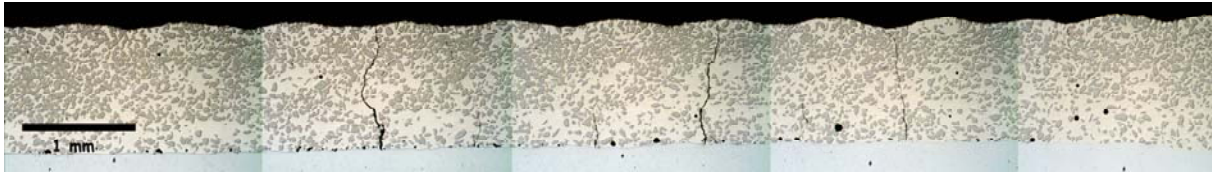
Figure 135. Regular wear pattern on the surface of laser clad Metco 12C + WC Woka 9604 (70/30 vol.%). Distance between the valleys is 1 mm.
