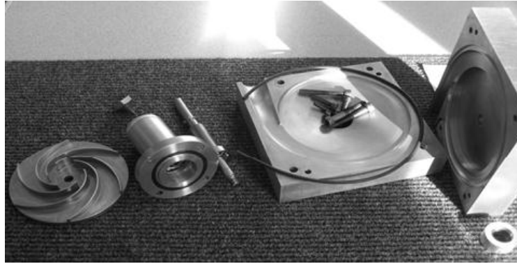
Figure 12. Example of a typical set of pump components manufactured by a student group (Childs et al. 2010, p. 5).
