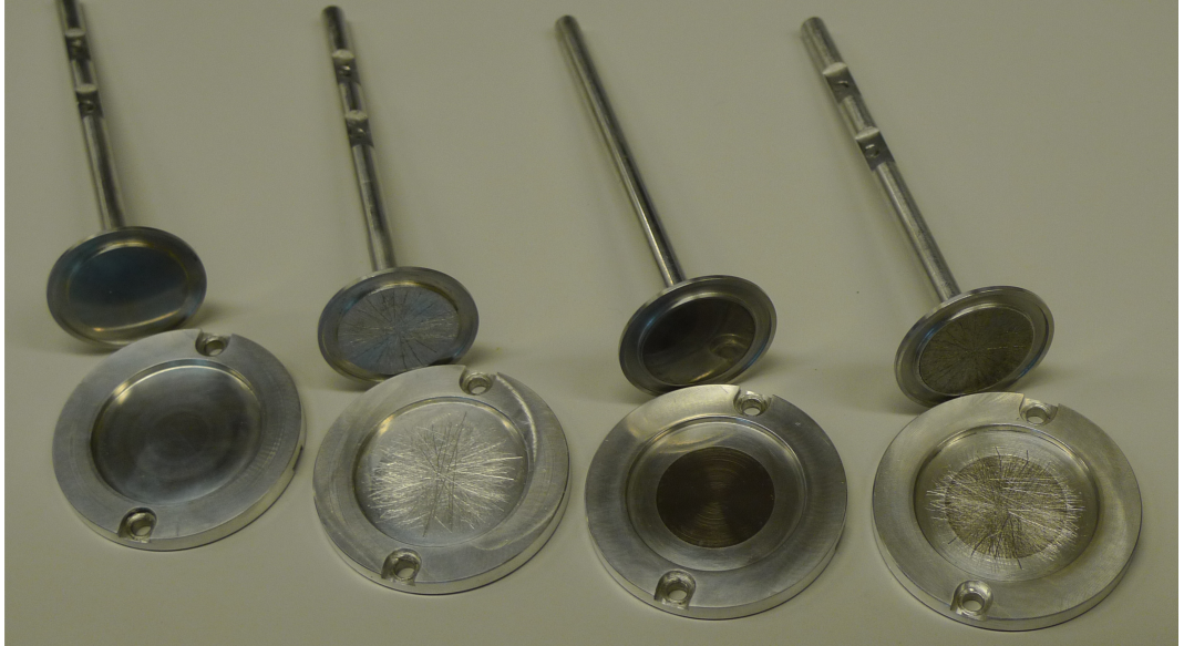
Figure 5.6: Custom plates from the left: smooth non-magnetic, rough non-magnetic, smooth magnetic, rough magnetic.
