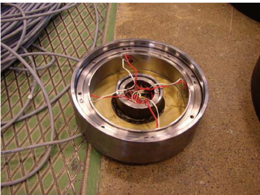
Figure 4.15 Assembly of earth pressure cell. The cell is shown without a front plate.
