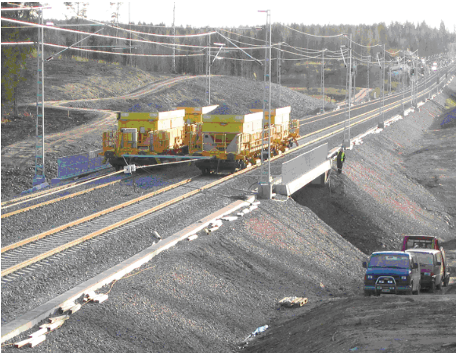
Figure 4.47 Field test arrangement at Tekemjärvenoja Railway Bridge (Koskinen et al 2005).
