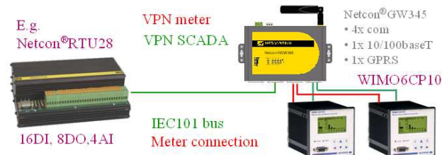
Figure 3. Monitoring and communication devices of a remote controlled secondary substation.
