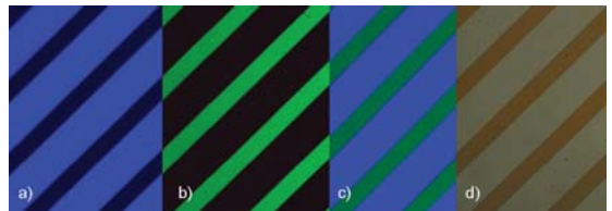
FIGURE 6 — Microscope image of the outcoupled light from the grating array: (a) blue LED on, (b) green LED on, (c) blue and green LEDs on, and (d) optical microscope image.
