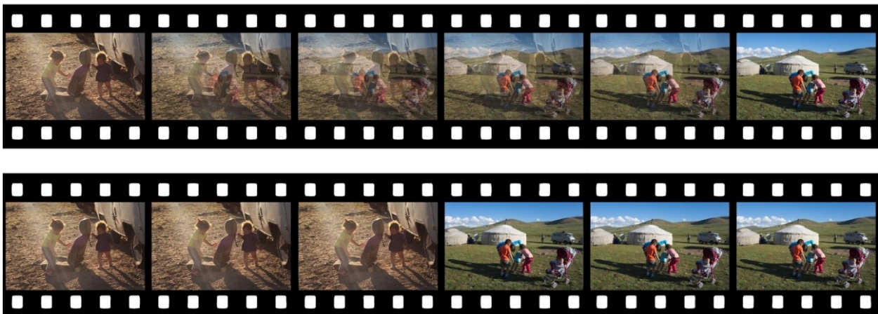
Figure 6-1. Gradual (above) and abrupt (below) shot changes in a video. Note that whereas it is easy to tell when the shot changes in an abrupt change, it is relatively hard to pinpoint when exactly the change occurs when shots are dissolved into each other.
