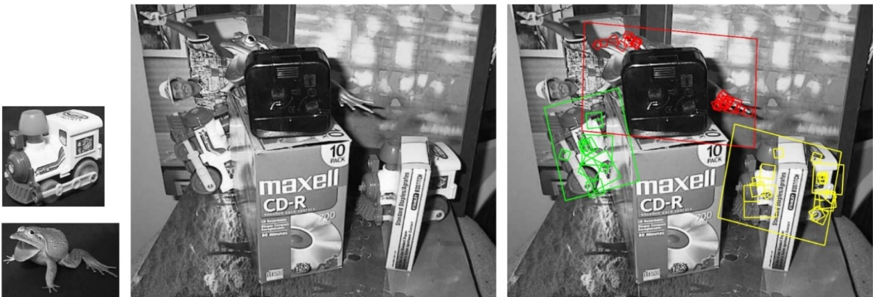
Figure 5-2. Object recognition via local image patches. Objects can still be detected despite occlusions, rotations and scale differences [83].
