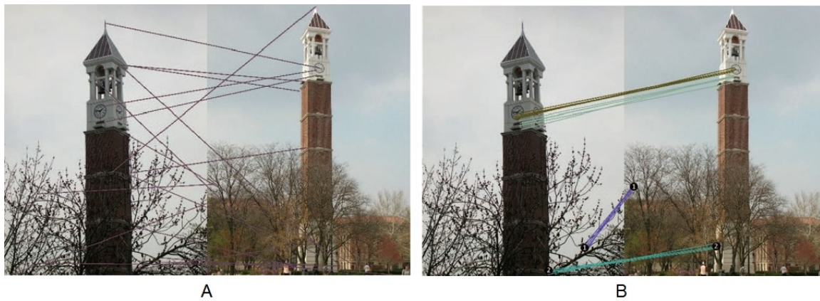
Figure 5-8. Local feature matching performance is usually affected by strong textured regions (A). Whereas neighborhood matching removes most of the incorrect matches, it is still possible to end up with erroneous results (B).
