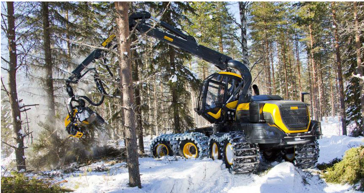
Figure 1. Example of a hydraulic boom on a modern forest harvester (at courtesy of Ponsse Ltd).
