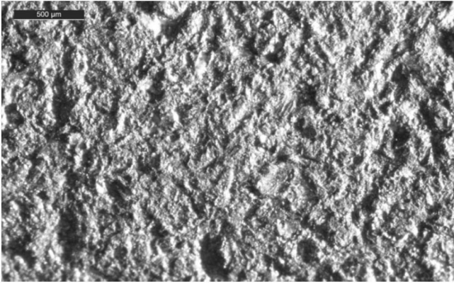
Figure 10. Wear surface of an AISI 316 sample.
