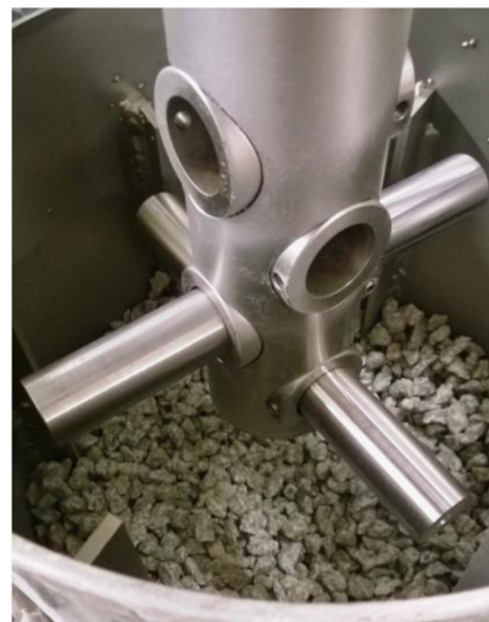
Fig. 2. Dry-pot test configuration for the erosion wear tests. Before the start of the test samples are submerged in to the abrasive bed. The shaft rotates anticlockwise during the test.
