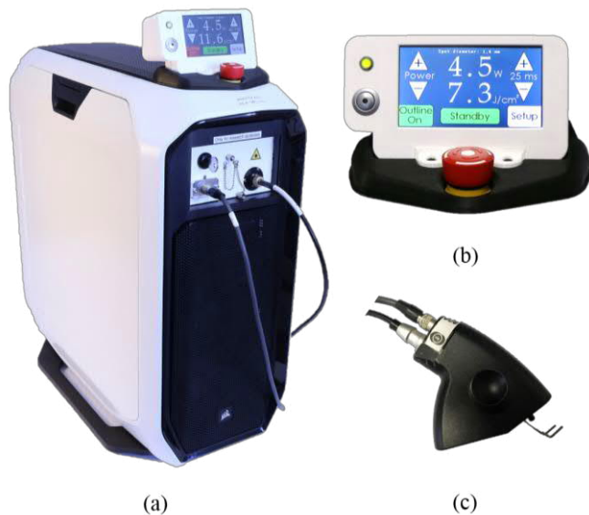
Fig. 5. Photo of the VECSEL module (a), the touch-screen on top with varied treatment parameters (b), and the MedArt handheld scanner (c).
