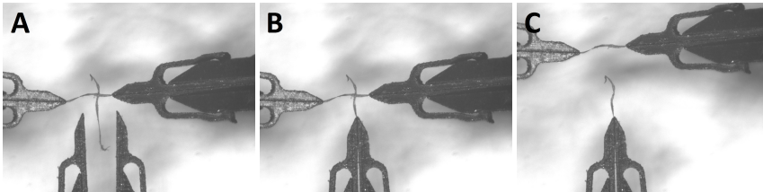
Figure 5.4: Shear-mode bonding force measurement process. (A) Microgrippers bring a fiber bond to the proximity of the PVDF based force sensing microgripper; (B) PVDF based force sensing microgripper grasps the free end of crossing fiber; (C) The microgrippers move away from the force sensing microgripper synchronously to break the bond.
