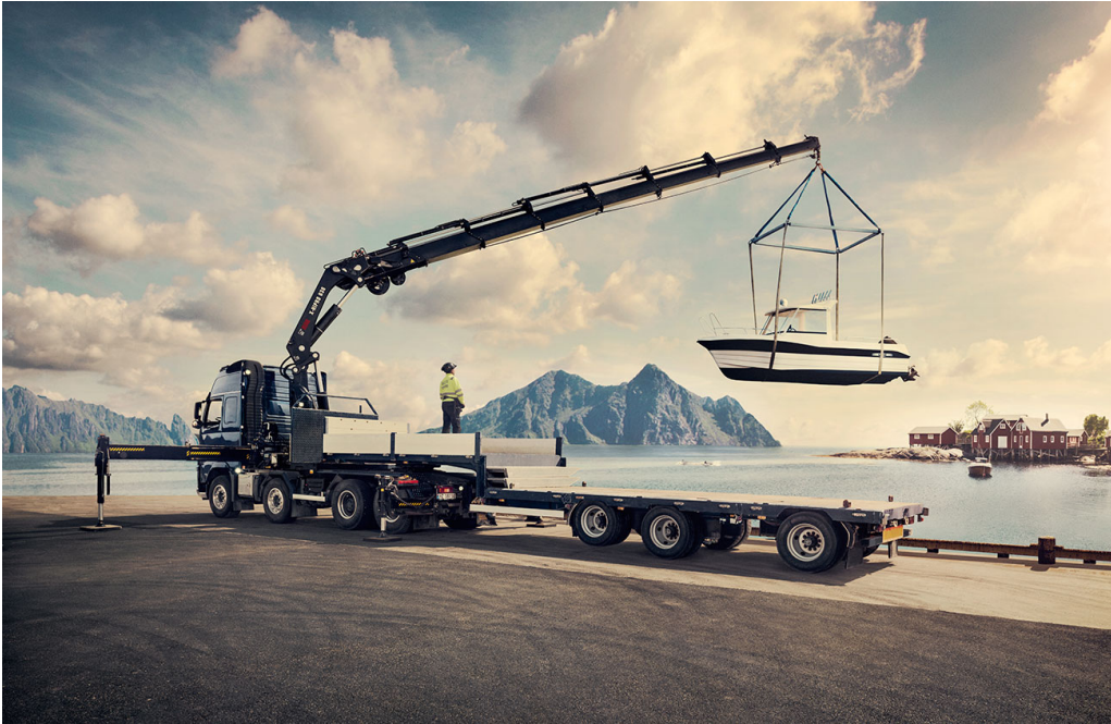
Figure 1.1: Heavy-duty hydraulic manipulator on a truck [1].
