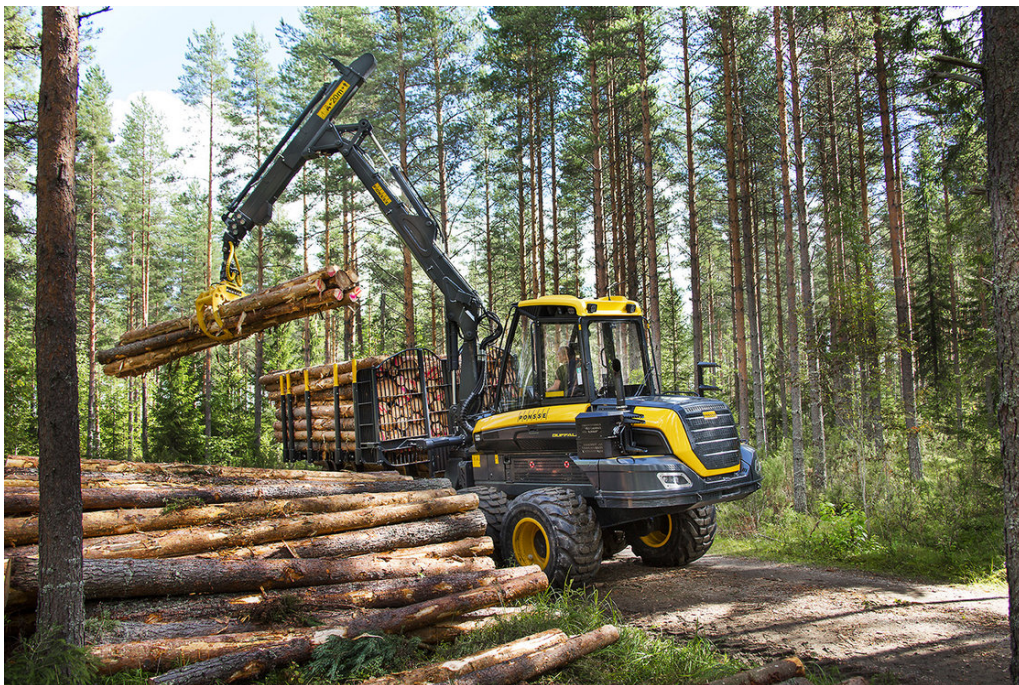
Figure 3.2: 4-DOF hydraulic manipulator on a forest forwarder [74].
