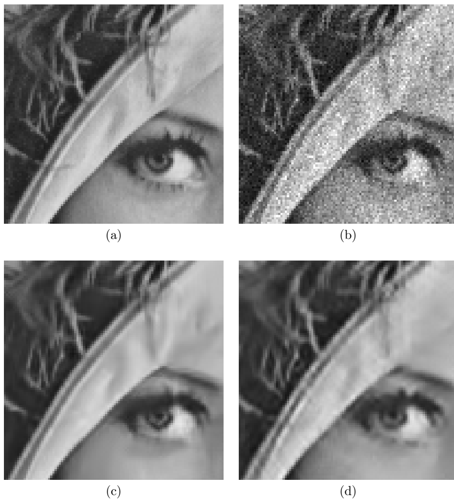
Figure 4.9: A 100 \times 100 section of each of the images in Figure 4.8. (a) Original image, (b) Noisy image (peak = 100, \sigma = 2 ), (c) Denoised with BM3D and the exact unbiased inverse \mathcal{L}_\sigma , (d) Denoised with UWT/BDCT PURE-LET.
