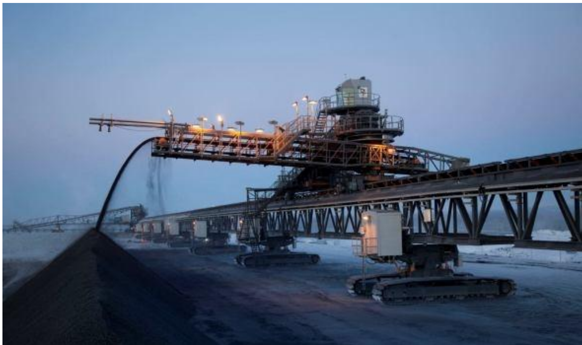
Figure 5.6. A crawler-mounted bridge stacker conveyor is an example product manufactured by Paakkola Conveyors (Picture: Paakkola Conveyors Ltd).
