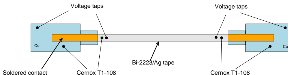
Figure 4.3: Voltage tap and temperature sensor locations over the soldered joint.
