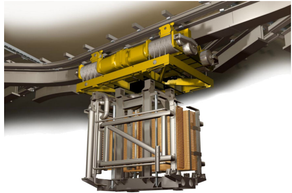
Figure 1.34: Main hoist attached to the monorail (image courtesy of CCFE)
