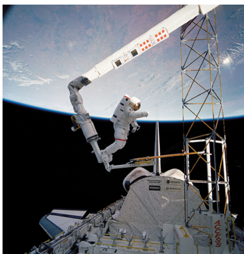
Figure 1.69: SRMS used as a platform for an extravehicular activity (image courtesy of NASA)
