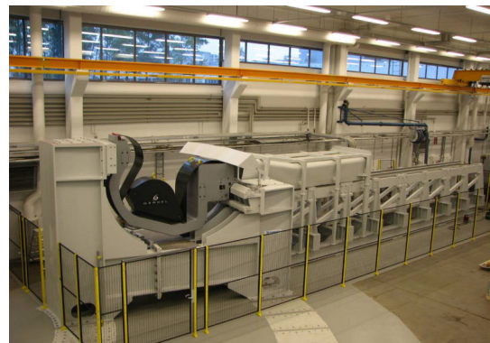
Figure 1.23: The full-scale divertor test platform DTP2, which is used for the design validation and demonstration of cassette operation capabilities (image courtesy of VTT-TUT)
