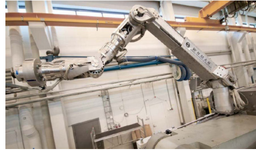
Figure 1.25: Demonstration of the manipulator arm mounted on the CMM at DTP2 (image courtesy of VTT-TUT)
