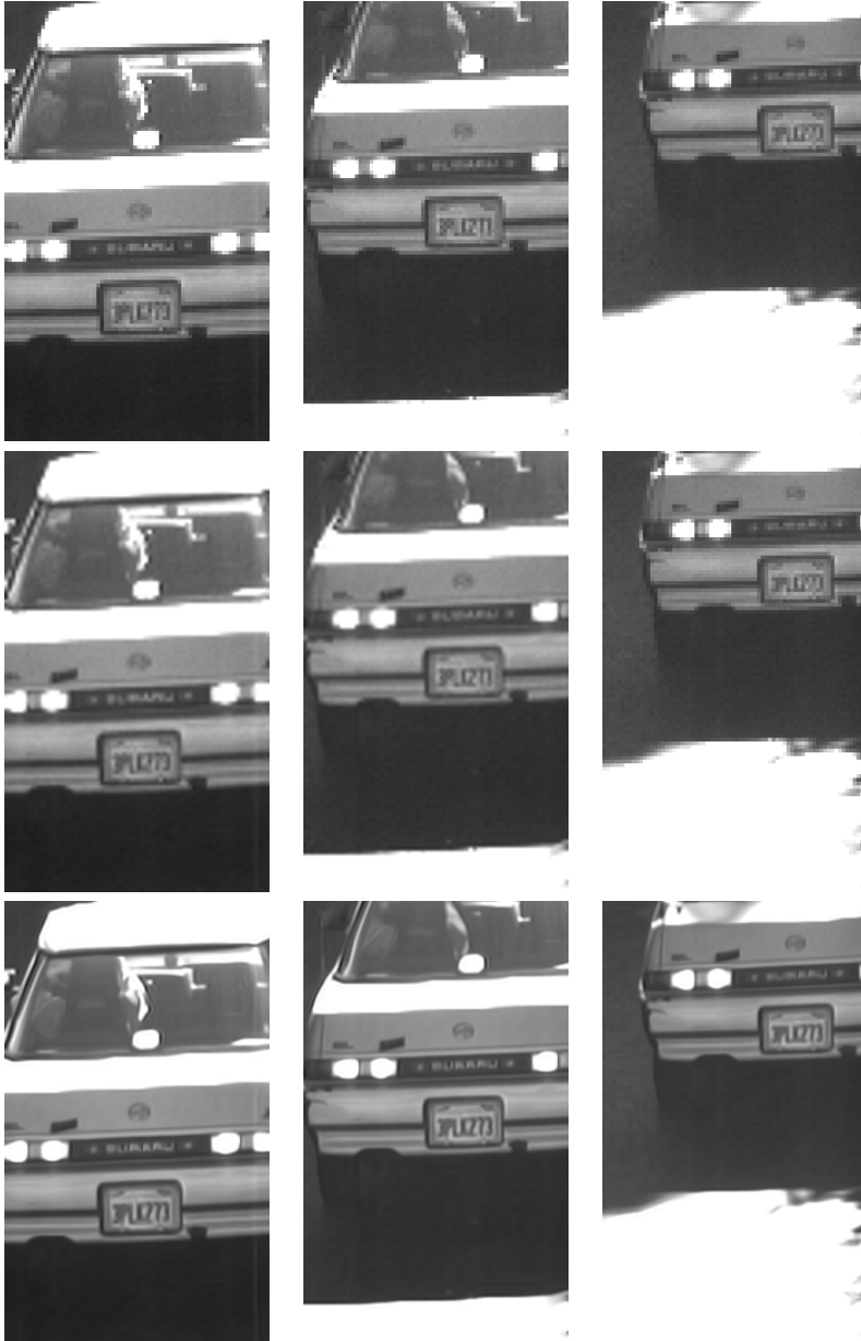
Figure 4.3: SR reconstruction from low-resolution video taken with infrared camera. The sequence contains in total 64 frames from which number 5, 30 and 60 are shown. From top to down: nearest-neighbour interpolation, bicubic interpolation, SR reconstruction with Algorithm 6. The images are 3 times larger the size of the LR images. The true degradation model is unknown; the model assumed by the reconstruction algorithm is 3 \times 3 uniform blur followed by decimation with factor 3.
