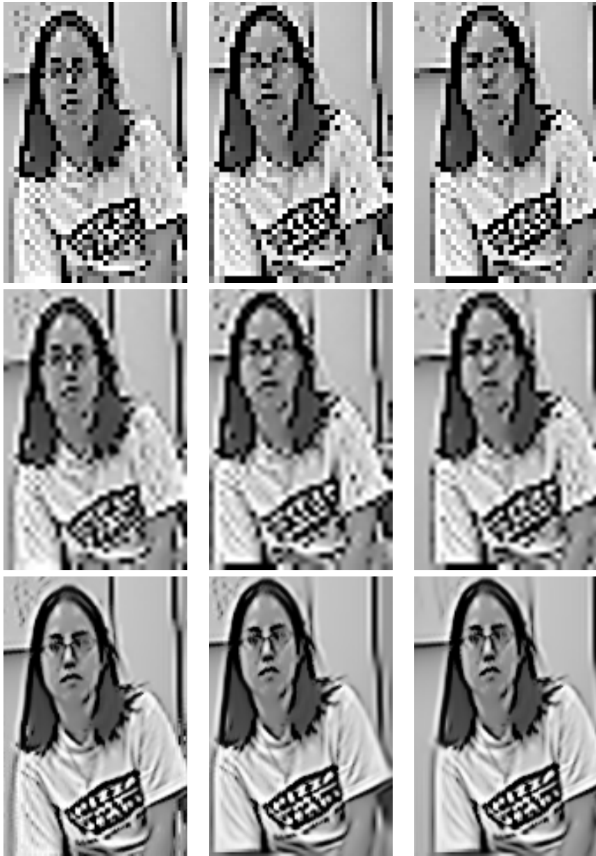
Figure 4.2: SR reconstruction from low-resolution compressed video taken with webcam. The sequence contains in total 53 frames from which number 10, 42 and 47 are shown. From top to down: nearest-neighbour interpolation, bicubic interpolation, SR reconstruction with Algorithm 6. The images are 3 times larger the size of the LR images. The true degradation model is unknown; the model assumed by the reconstruction algorithm is decimation with factor 3, no blur ( \mathbf{A} = \mathbf{I} ).
