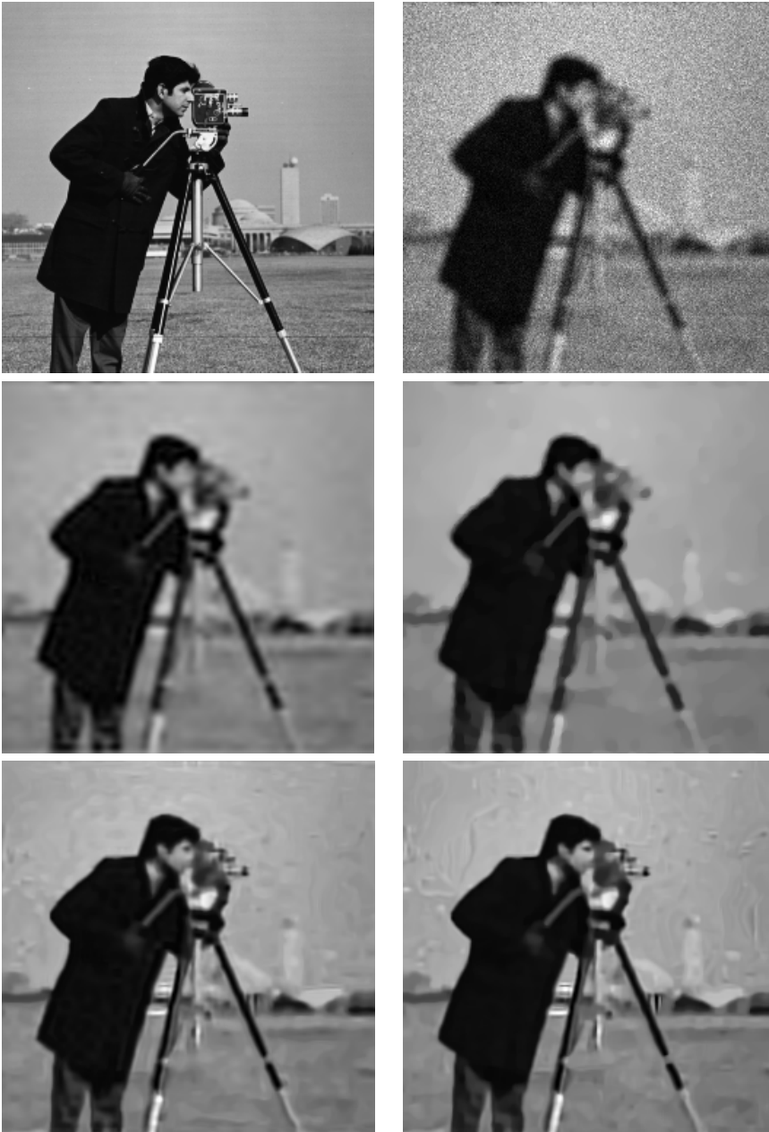
Figure 3.6: Deblurring of the Cameraman image, scenario 3. From left to right and from top to bottom are presented the following images: original, blurred noisy, reconstructed by DFS[DFS09] (PSNR 21.59, MAE 4.75), PIDAL-TV[FBD10] (PSNR 22.03, MAE 4.07), PIDD-BM3D with constructing frames using the result of DFS (PSNR 23.32, MAE 3.73), PIDD-BM3D with constructing frames using the result of PIDAL-TV (PSNR 23.49, MAE 3.59).
