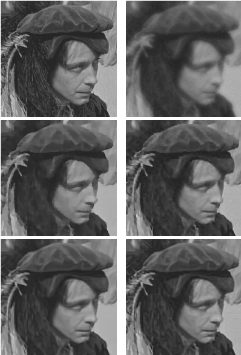
Figure 3.3: Deblurring of the Man image, scenario 2. From left to right and from top to bottom are presented zoomed fragments of the following images: original, blurred noisy, reconstructed by CGMK [CGMK10] (ISNR 4.34), L0-AbS [Por09] (ISNR 4.42), DEB-BM3D [DFKE08a] (ISNR 4.82) and by proposed IDD-BM3D method (ISNR 5.12).
