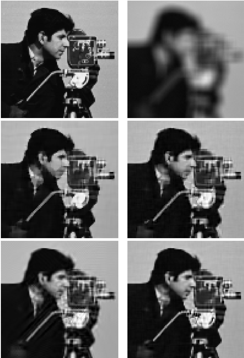
Figure 3.2: Deblurring of the Cameraman image, scenario 3. From left to right and from top to bottom are presented zoomed fragments of the following images: original, blurred noisy, reconstructed by CGMK [CGMK10] (ISNR 9.15), L0-Abs [Por09] (ISNR 8.96), DEB-BM3D [DFKE08a] (ISNR 8.37) and by proposed IDD-BM3D method (ISNR 10.48).
