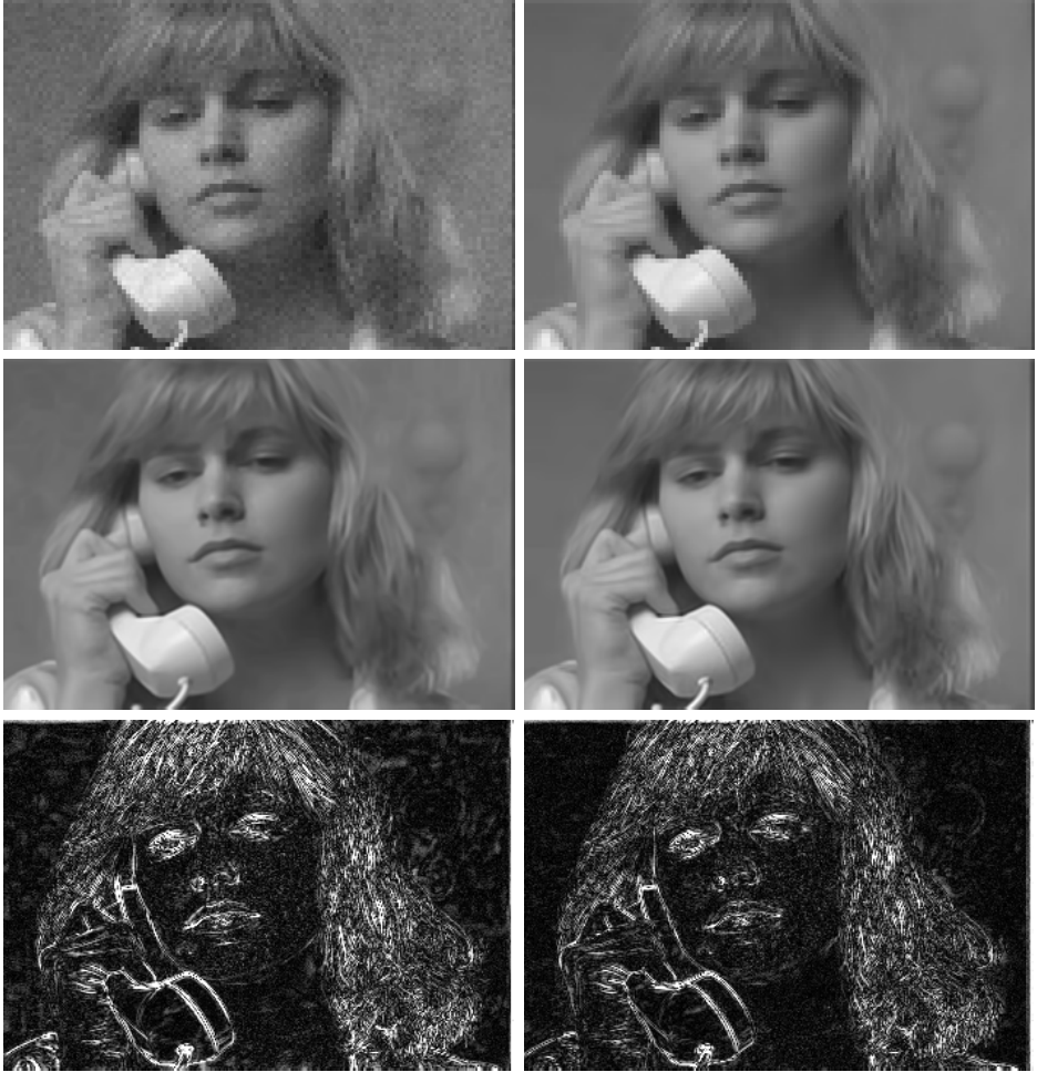
Figure 4.4: Comparison of two reconstruction approaches: directly from noisy and from prefiltered data. The synthetic LR sequence is obtained from the original HR sequence Suzie by blurring frames with 3 \times 3 uniform PSF, decimating with factor 3 and adding AWGN with \sigma = 5 . The test sequence contains 30 frames; frame number 21 is shown. Top row: nearest-neighbour interpolation of noisy frame, nearest-neighbour interpolation of prefiltered frame. Middle row: reconstruction with Algorithm 6 directly from noisy data ( \gamma = 0.3, \tau_{dc} = 91.1, \tau_{ac} = 1053 , mean PSNR over 30 frames 32.4 dB), reconstruction with Algorithm 6 from prefiltered data ( \tau_{dc} = 14.6, \tau_{ac} = 1053 , mean PSNR over 30 frames 33.1 dB). Last row: differences between the reconstructed and ground truth images.
