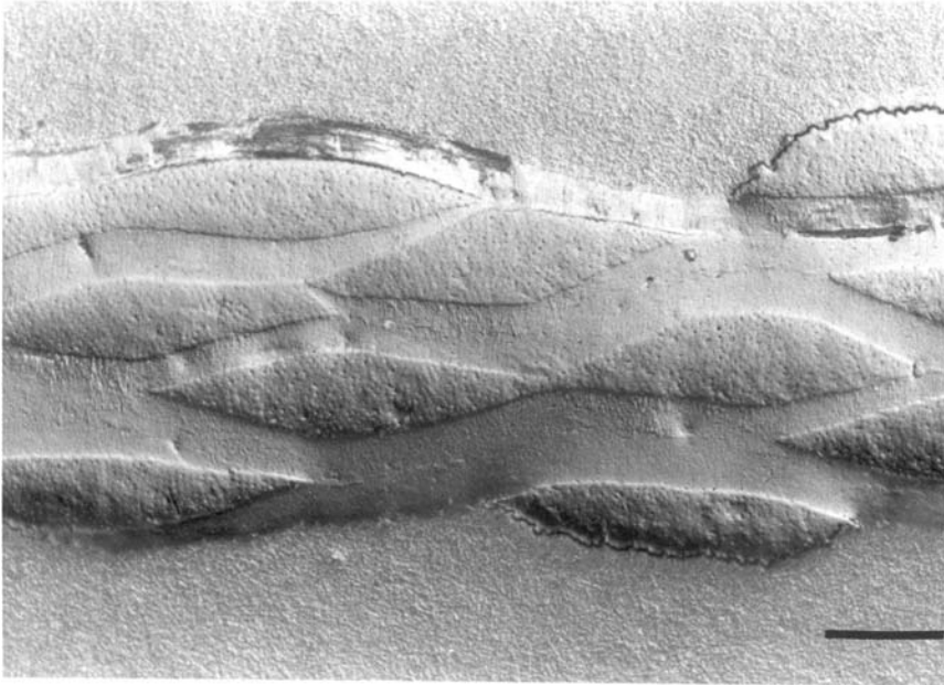
Figure 10. Polished cross-section of single sandwich system. 5 standard woven fibre layers + HAPEX™. Cursor = 200 \mu\text{m} .
