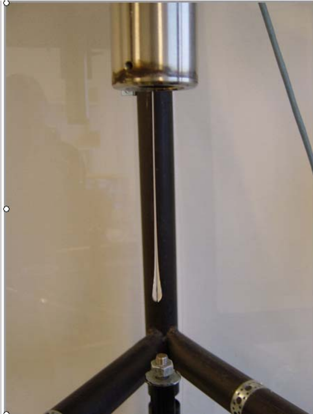
Figure 15. Photograph of bioactive glass drop, slowly falling down from the glass melt.
